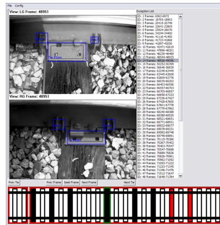
Figure 10. Our exception visualization tool shows the consolidated results: A black tie indicates a tie with complete boxed anchors (4 anchors), a red tie indicates a tie with incomplete boxed anchors (1-3 anchors), and a white tie has 0 anchors.
