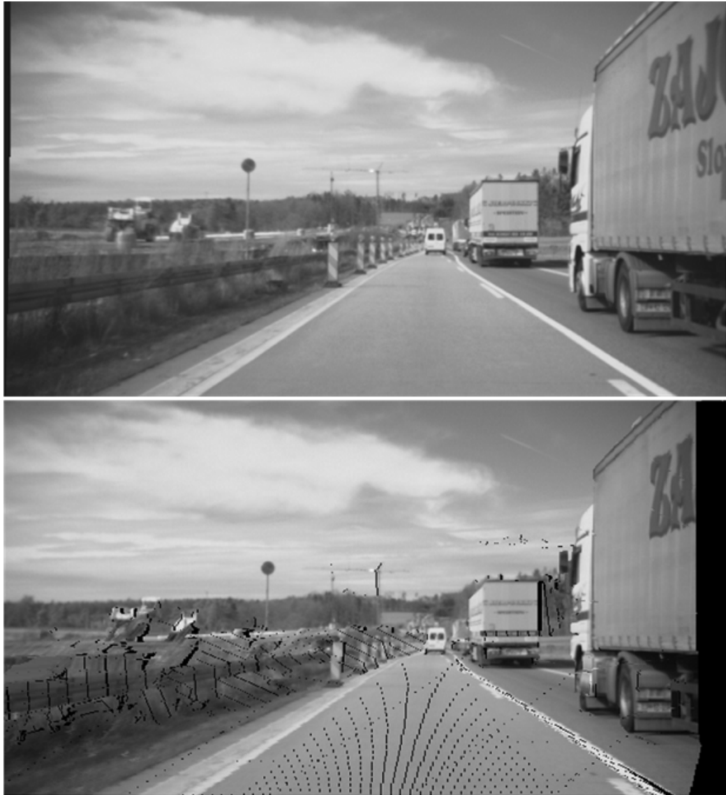
Figure 6.4: Top: original fourth frame I_R^{t+1} . Bottom: predicted fourth frame \hat{I}_R^{t+1} . The black pixels are missing values caused by bilinear interpolation. These pixels are excluded when computing the view prediction error.
