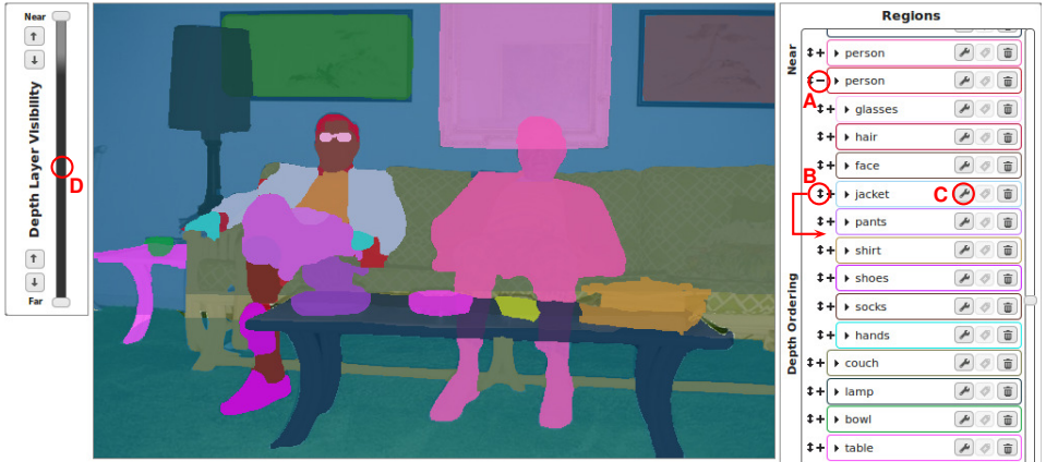
Figure 3: Annotation interface. Our web-based image annotation tool renders partially transparent color-coded regions (center) according to the occlusion order determined by their position in the tree (right panel). The right panel serves as a graphical interface for controlling the level of detail displayed by expand/collapsing nodes (A). More importantly, it enables rearrangement of tree structure by clicking and dragging nodes to different locations in the tree (B). Here, the user should correct the ordering of jacket and pants by dragging jacket to be behind (occluded by) pants. Buttons next to each region (C) swap to the region editing mode detailed in Figures 4 and 5. The slider in the left panel (D) peels off occlusion layers, allowing quick visualization of global figure/ground structure.
