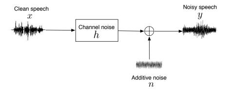
Figure 6.1: The relationship between clean speech x, additive and channel noise (n, h)and noise corrupted speech y.
