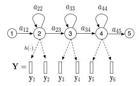
Figure 2.5: Topology of a 5-states left-right HMM with 3 emitting states and 2 non-emitting states. State 1 is the entrance state and state 5 is the exit state and both of them are non-emitting.  $a_{ij}$  denotes the state transition probability from state i to state j.  $b(\cdot)$  is the density function.
