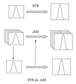
Figure 6.3: A comparison of VTS and JUD noise compensation. VTS is performed on per component basis, while for JUD, a cluster of components share the same compensation parameters.
