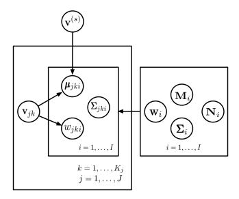
Figure 3.1: Model structure of a SGMM acoustic model, with total J HMM states, and each has  $K_j$  sub-states. Each sub-state is modelled by a GMM with I components, whose parameters are derived from  $\Phi_i = \{\mathbf{M}_i, \mathbf{N}_i, \mathbf{w}_i, \mathbf{\Sigma}_i\}$  and  $(\mathbf{v}_{jk}, \mathbf{v}^{(s)})$  using Eq. (3.2) and (3.3), and for covariance  $\mathbf{\Sigma}_{jki} = \mathbf{\Sigma}_i$ .
