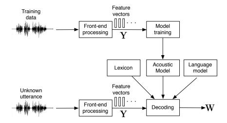
Figure 2.1: Diagram of a standard speech recognition system.
