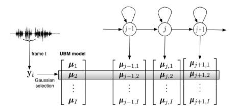
Figure 3.2: An example of Gaussian selection using UBM model. For each acoustic frame  $\mathbf{y}_t$ , the UBM is used to select the active Gaussian components in the SGMM acoustic models. For instance, in this figure, the second Gaussian represented by  $\boldsymbol{\mu}_2$  is among the top P Gaussian components according to its likelihood score for  $\mathbf{y}_t$ , thus all the second Gaussian in each SGMM sub-state is active for this frame.
