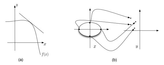
Figure 6.6: A comparison between VTS and UT approximation: (a) VTS approximates the nonlinear function y = f(x) by vector Taylor series expansion, and results in a linear function by using first order VTS. (b) UT draws sigma points from the distribution of x and synthesise the corresponding samples of y by the nonlinear function f(x).
