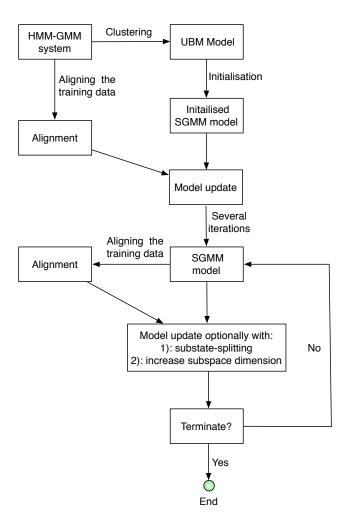
Figure 3.3: Block-diagram of SGMM acoustic model estimation.
