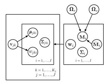
Figure 5.2: MAP adaptaion of  $\mathbf{M}_i$  in SGMM acoustic model.  $(\bar{\mathbf{M}}_i, \mathbf{\Omega}_r, \mathbf{\Omega}_c)$  denote the hyper-parameters of the Gaussian prior  $P(\mathbf{M}_i)$ , in which the mean  $\bar{\mathbf{M}}_i$  is indexed by I while the covariances  $\mathbf{\Omega}_r$  and  $\mathbf{\Omega}_c$  are global.
