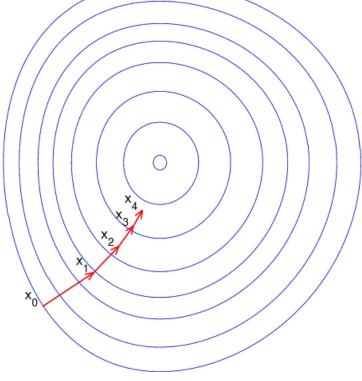
minimizes a function F by taking steps in proportion to the negative of the gradient:
