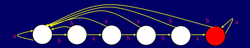
Combination-lock automaton: basically simulating a conjunction.
